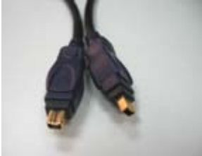
Connecting a 4-pin to 4-pin IEEE-1394 cable to a notebook computer
