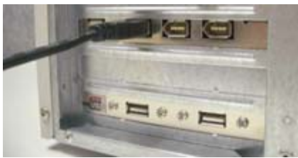
Connecting a 4-pin to 6-pin IEEE-1394 cable to a desktop computer
