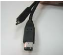
Connecting a 4-pin to 6-pin IEEE-1394 cable to a desktop computer
