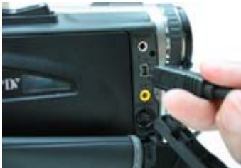
Connecting the IEEE-1394 cable to the DV camcorder
