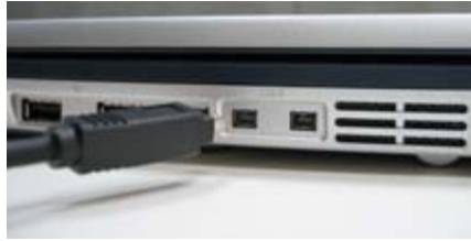
Connecting a 4-pin to 4-pin IEEE-1394 cable to a notebook computer
