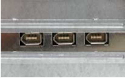
6-pin IEEE-1394 ports on a desktop computer
