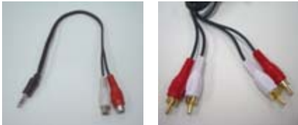
Line-in and audio cables for S-Video
