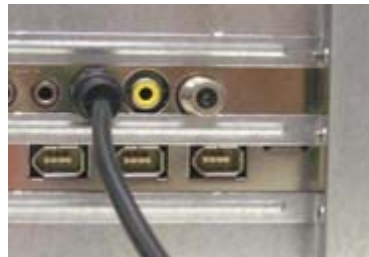
Connecting the S-Video source to the capture card
