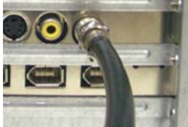
Connecting TV antenna to the tuner card
