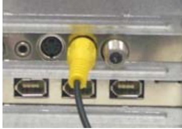
Connecting the Composite video source to the capture card
